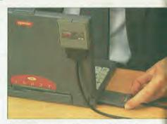
Olivetti has developed a DECT-based PC Card with a small-stub antenna for use with wireless LANs. The Net3 clients use a PC Card that emulates an Ethernet or Token Ring card and a detachable aerial that can be positioned apart from the notebook.
